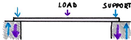
When a single beam spans any distance, the very top of the beam gets the most compression, and the very bottom of the beam experiences the most tension. The beam needs to be strong to resist these forces. You also need to apply weight at both ends to counteract the bending at the centre.
