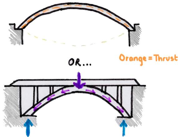
The semi-circular structure distributes compression through its entire form and diverts weight onto its two abutments, the part of the bridge that directly take on pressure. It needs firm foundations, to allow all the parts to push back against each other.
